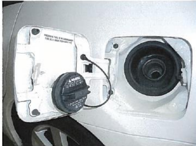
Figure 6-13. Example of an error-proofing device: a gas cap strap
