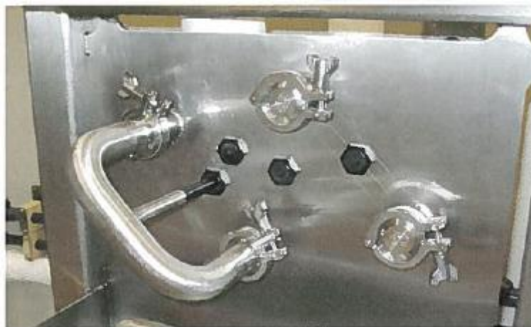
Figure 6-14. Example of error-proofing device used in biomanufacturing
